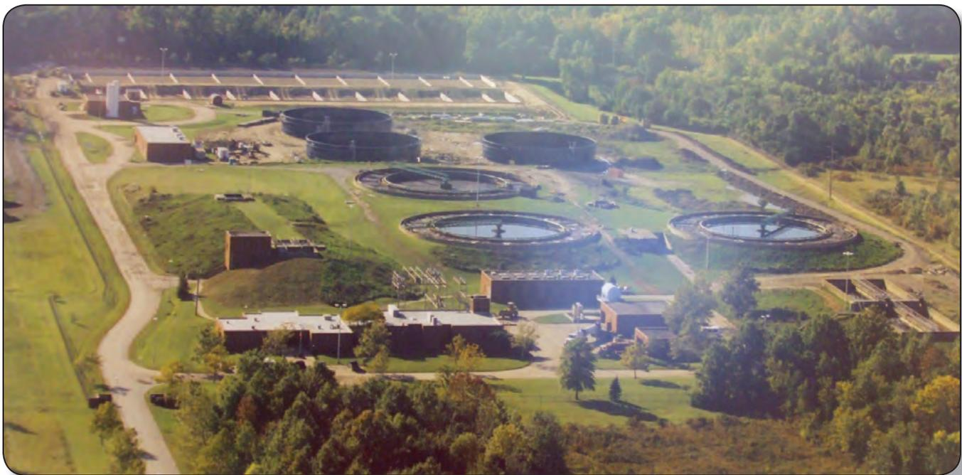
*Aerial view of French Creek Wastewater Treatment Plant in 1996. Administration Building at lower left, Grit Building at center left, Sludge Building at upper left, and clarifier tanks at center right (City of North Ridgeville).*
