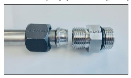
Typically, medium to heavy wall tubing is used in flareless application. Minimum wall for tubing used with flareless fittings ranged from .028" to .095", depending on tube OD. Tubing made from 304 or 316 stainless steel may be welded, seamless or DOM (Drawn over Mandrel) that is annealed.
