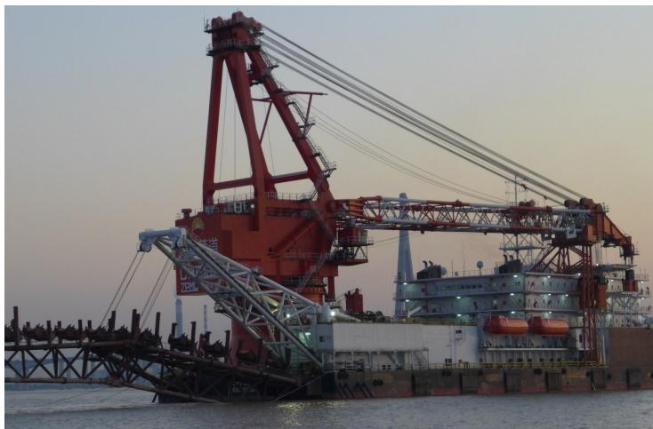
The Pipe Lay Barge is equipped with 8 Mooring Winches and 2 Anchor Winches (130 ton Winches). Each Winch uses Logan CH 2150 Hydraulic Actuated, Air Cooled Clutch for Winching In and Pay Out operation. Controlled remotely from the wheel house or local engagement.
