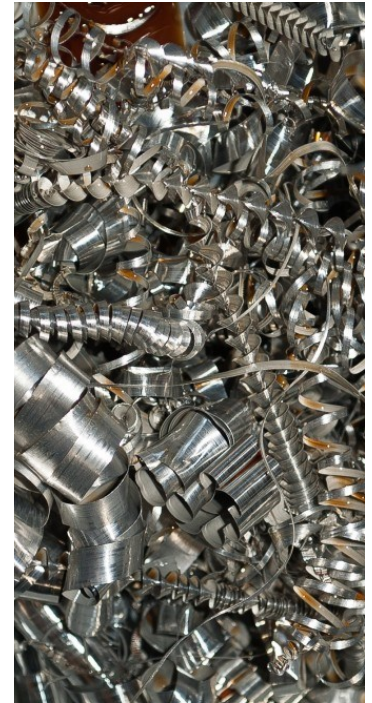
Aluminum 6061 raw material stringers from a sample job on an 1 3/4"-6 Wickman.
