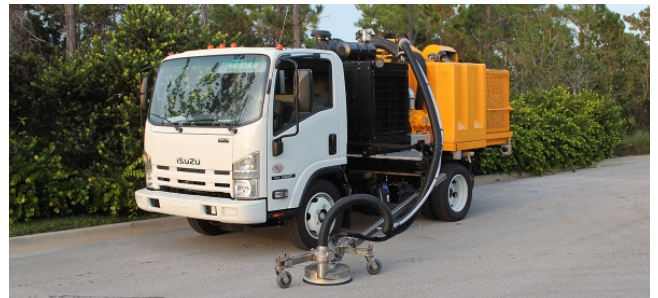
Medium Duty surface preparation truck equipped with Logan LC-211 Bell Housing PTO powered by a 200 HP Diesel engine.
