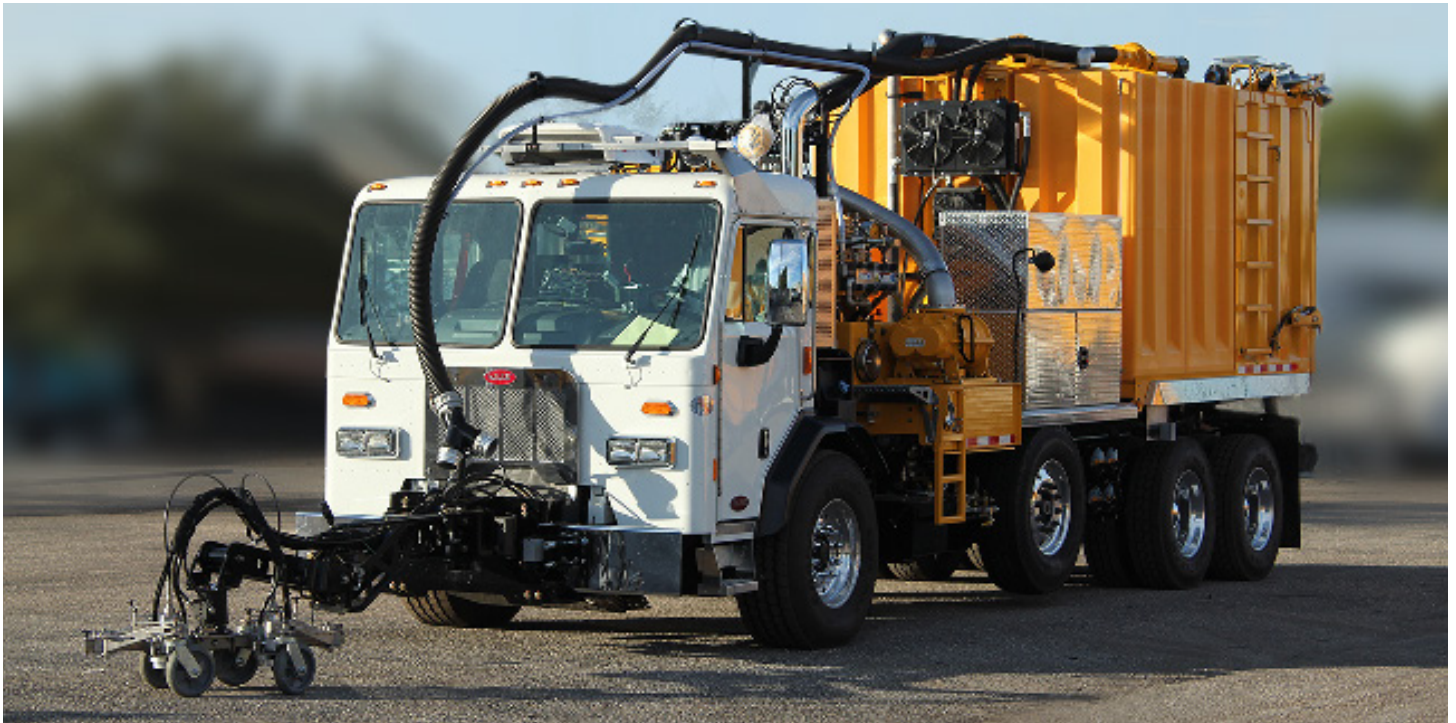
Waterblasting truck equipped with 375 HP Diesel Engine and an air / fluid actuated Logan LC-314 Bell Housing PTO for smooth engagement.
