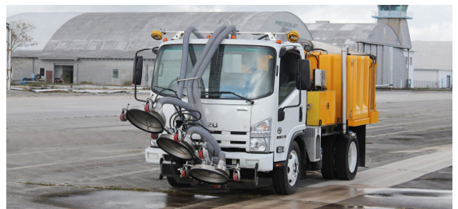
Heavy duty airport marking removal truck equipped with a Logan LC-311 Bell Housing PTO, with SAE No. 3 flywheel mount, powered by a 240 HP diesel engine.
