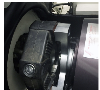
A flexible coupling dampens the torsional vibrations between the Scania 405 and the Logan SPF 1000 Series
