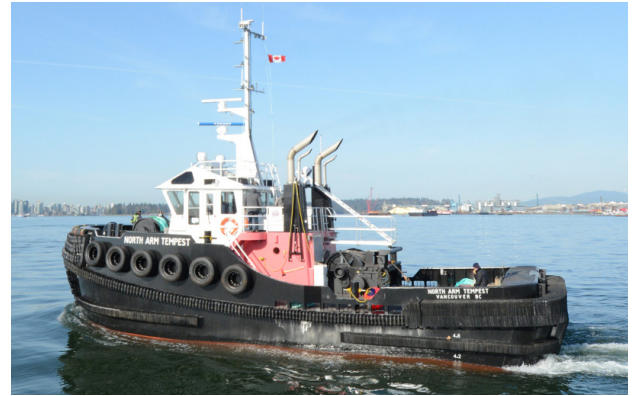
The North Arm Tempest uses SPF-600 series Logan Front of Engine Power Take-off clutches to provide on-demand connect/disconnect power from the John Deere 4045TFM85 engines to Kawasaki pumps that power the hydraulic systems
