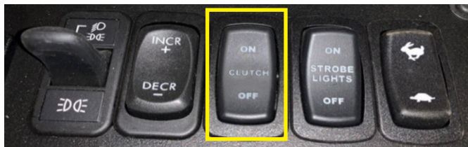
Clutch can be controlled by a remote switch in the cab or by a switch at the Power Pack
