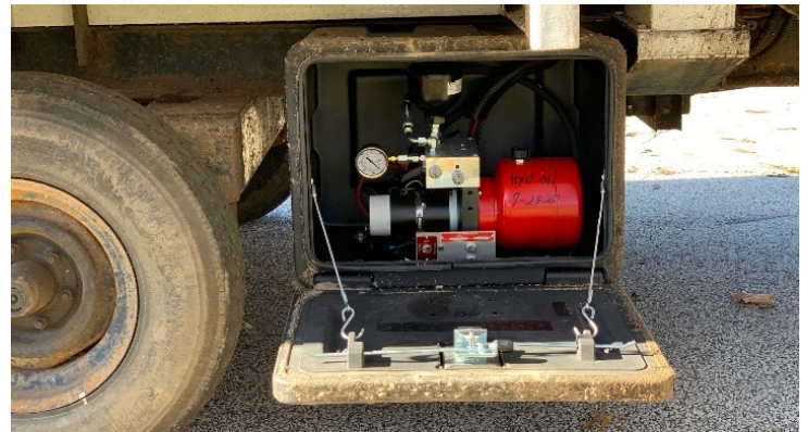
Logan Hydraulic Power Pack with Softstart™ actuation for smooth engagement
