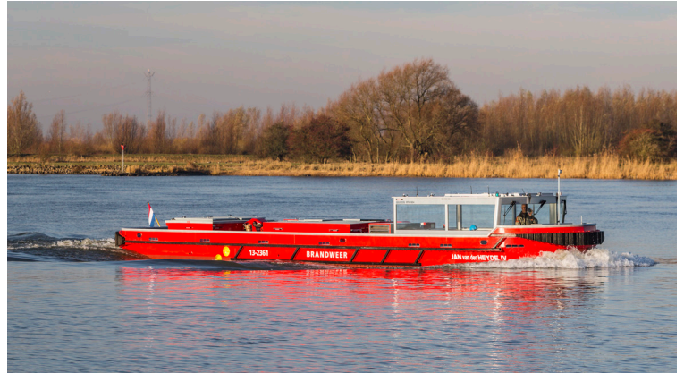
The Jan van der Heyde's low profile design allows it to pass underneath Amsterdam's Canals and bridges to provide overwhelming water flow in fire emergencies
