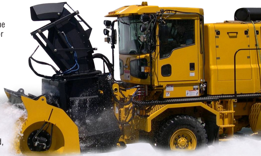
OshKosh H-Series Snow Blower Truck with Logan Bell LC-314 Bell Housing PTO Clutch
