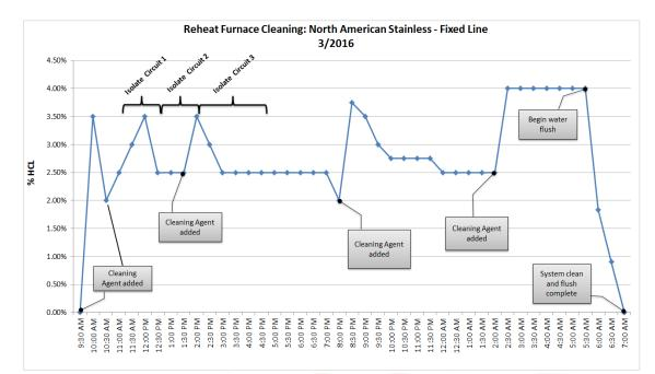
Figure 2: Graph of cleaning process for Cooling Water System, NAS
