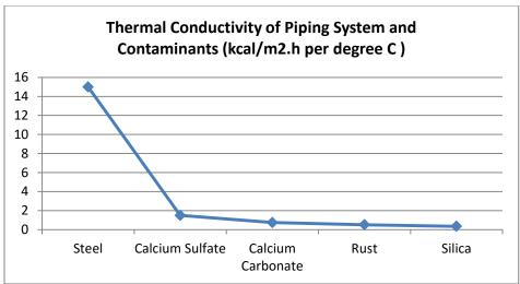
Figure 1: Thermal conductivity of steel and water contaminant buildups
